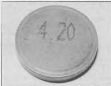
15.13 Shim thickness is marked on the lower face (here 4.20 mm)
