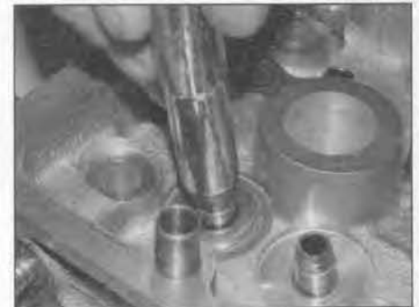
8.2 Use a suitable socket or metal tube to press the valve stem oil seal firmly onto the guide
