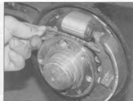
8.8b ... then lift out the self-adjuster mechanism
