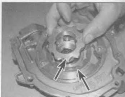
15.10 After inspection, refit the pump rotors with the orientation marks (arrowed) facing upwards
