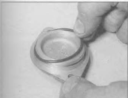
10.22a Locate a new O-ring on the inlet camshaft cover plate ...
