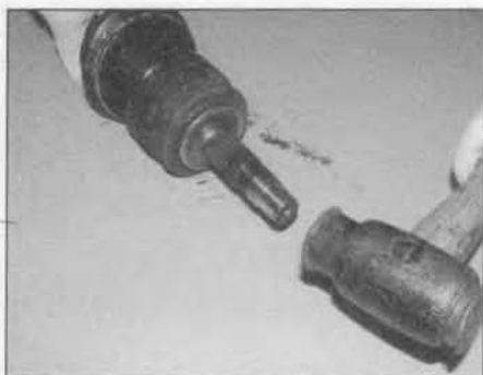
3.13b . . . then tap the joint onto the shaft until the circlip engages
