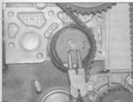
5.23 Using right-angled circlip pliers, turn the tensioner pulley to fully tension the belt
