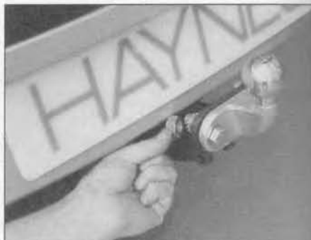
28.22 Secure the fixed towball to the towbar neck flange with the two bolts nuts and lockwashers
