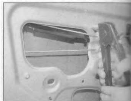
16.33 Refit the anti-theft partition and secure with new pop rivets
