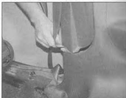
25.36 Slide the seat belt out through the incision in the panel – 3-door models
