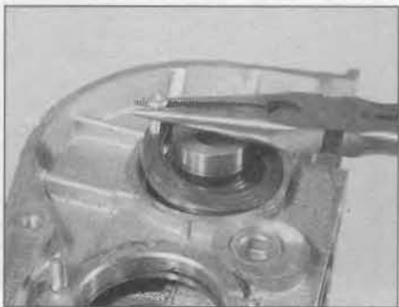
10.10 Extract the exhaust camshaft oil seal ...
