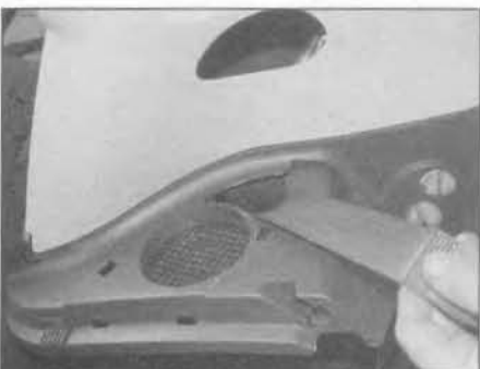
25.54 ... then withdraw the seat belt through the incision in the loudspeaker housing
