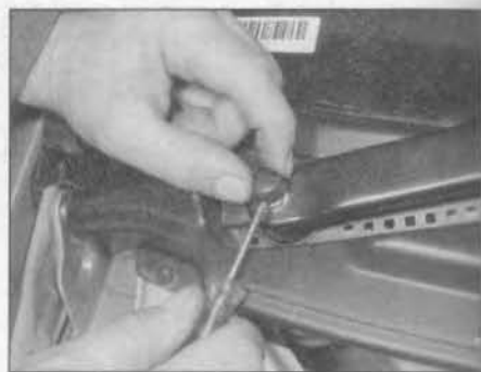
17.3 Prise off the wiper arm spindle nut cover, then slacken and remove the spindle nut
