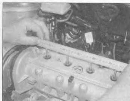
5.13 Place a straight-edge along the top of the rods and turn the crankshaft until the straight-edge contacts all four rods
