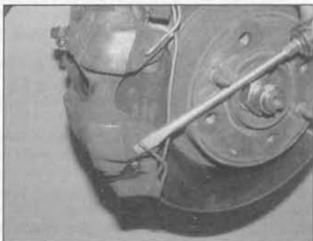
4.5 Prise the lower end of the pad retaining spring clip from the caliper body – DOHC (16-valve) engine models
