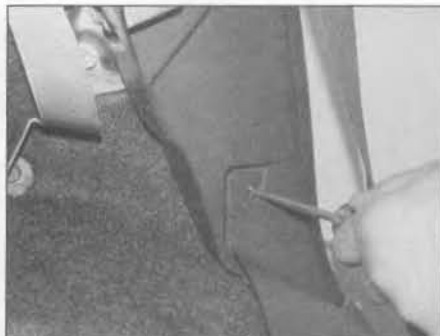
25.43 Undo the screw securing the upper corner of the panel above the wheel arch – 5-door models
