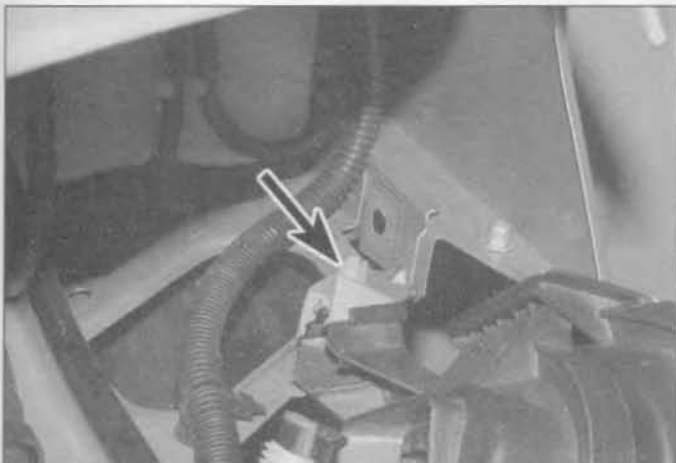
6.3b ... then disengage the locating peg (arrowed) from the front wing
