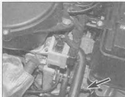
24.2 Manual transmission oil filler/level plug location (arrowed)
