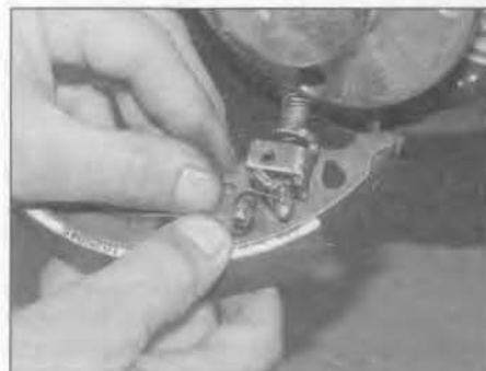
8.10 Lift the locking catch on the trailing shoe handbrake lever, and slide out the handbrake cable end
