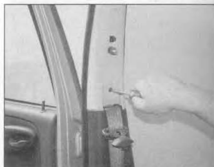
25.25 Undo the retaining screw at the base of the centre pillar trim panel upper section – 5-door models
