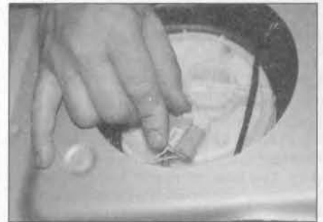
6.5 Release the locking catch and disconnect the wiring connector from the fuel pump
