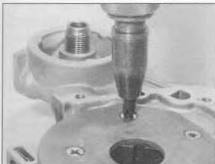
15.9 Using an impact screwdriver to remove the oil pump rear cover plate screws
