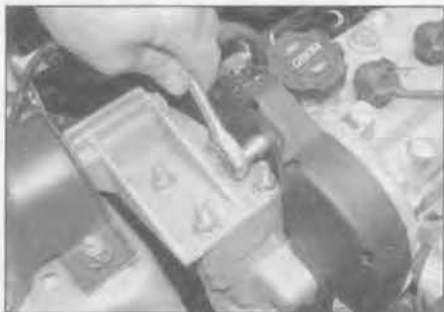
4.3a Undo the timing belt upper cover retaining bolt above the engine mounting ...
