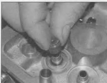
6.8a Extract the valve stem oil seal from the top of the guide ...
