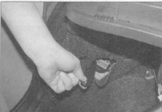
4.31 Fold back the carpet access flap and unscrew the lower securing bolt in the same way
