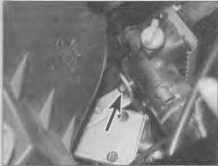
3.7 Undo the bolt (arrowed) securing the automatic transmission fluid heat exchanger to the radiator
