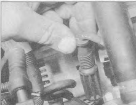
A Check that the spark plug HT leads are securely connected at the spark plugs ...
