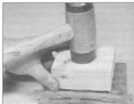
17.10c ... and use a block of wood to drive it in - SOHC (8-valve) engines
