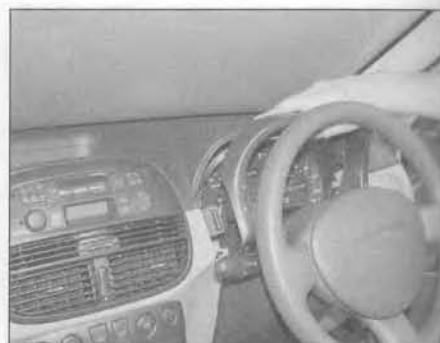
27.11b ... then withdraw the surround from the fascia
