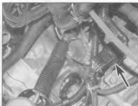
4.12a Disconnect the main wiring harness connector (arrowed) at the top of the transmission . . .
