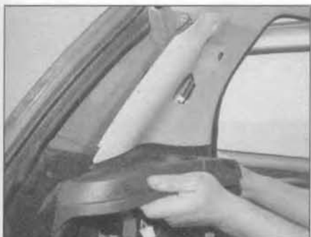
25.53 Carefully pull the support away from the body to release the securing clips ...
