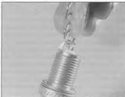
16.9 Adjusting a spark plug electrode gap
