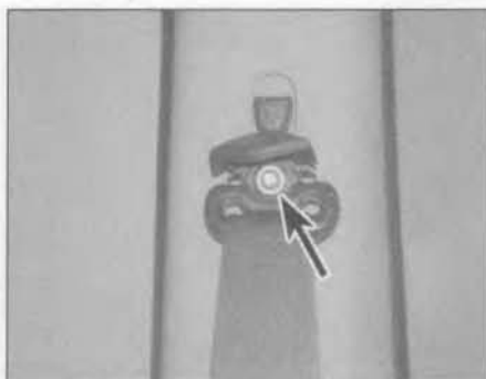
24.3 Front seat belt upper anchor nut (arrowed)
