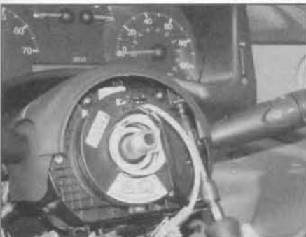
27.8a Undo the two screws securing the front of the upper shroud to the switch assembly ...
