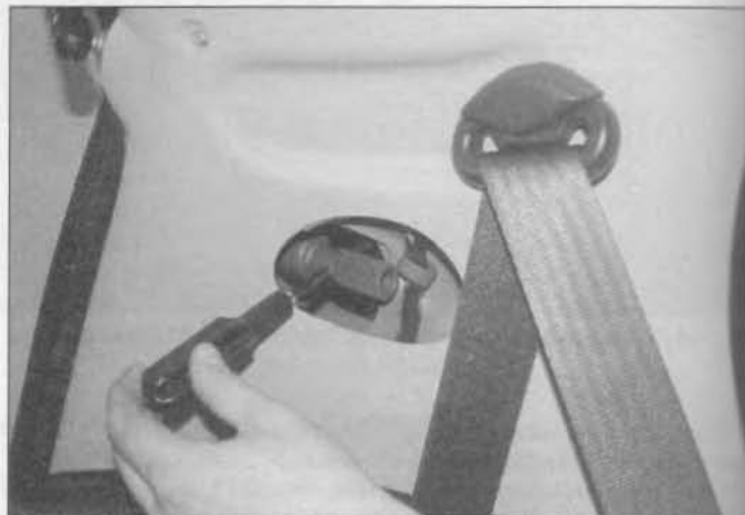
4.30 Unscrew the rear light cluster upper securing bolt using the screwdriver and special socket
