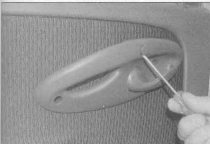
14.16a Lift off the trim caps and undo the retaining screws . . .
