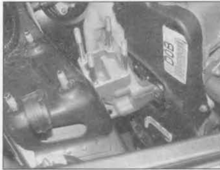
4.6 Undo the four bolts and remove the right-hand mounting lower bracket from the cylinder head
