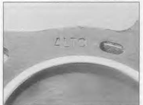
11.19 Place the cylinder head gasket on the block so that the word ALTO can be read from above
