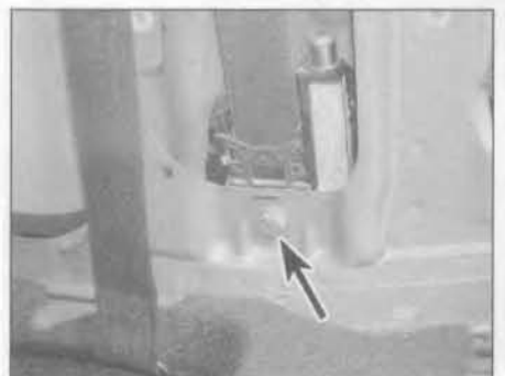
24.4 Front seat belt inertia reel retaining bolt (arrowed)
