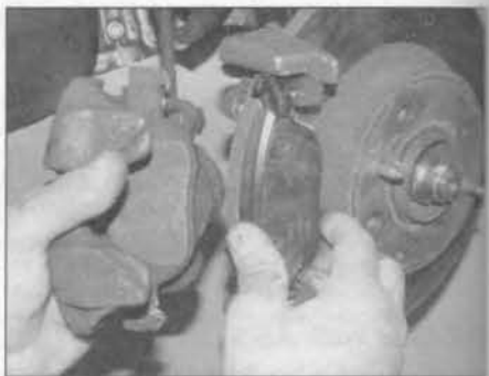
4.9b . . . and withdraw the outer brake pad from the mounting bracket – DOHC (16-valve) engine models
