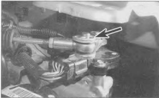
2.3a Extract the selector cable end fitting retaining clip (arrowed) . . .
