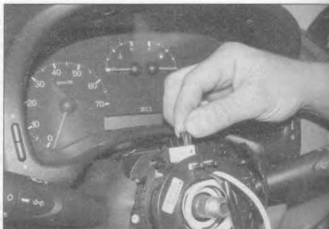
20.12 Disconnect the wiring connector from the top of the airbag clockspring
