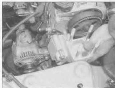
5.9b ... and remove the right-hand mounting lower bracket from the cylinder head
