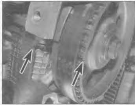
2.12a Camshaft sprocket and cylinder head TDC timing marks (arrowed) aligned
