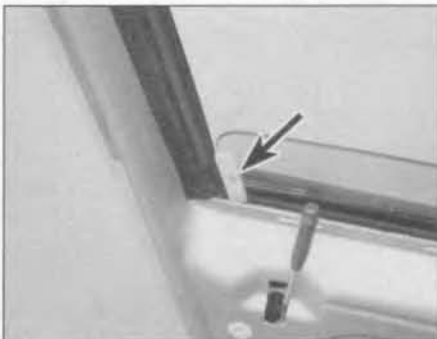
18.6 Pull the glass out of the rear guide channel to disengage the plastic slider (arrowed)
