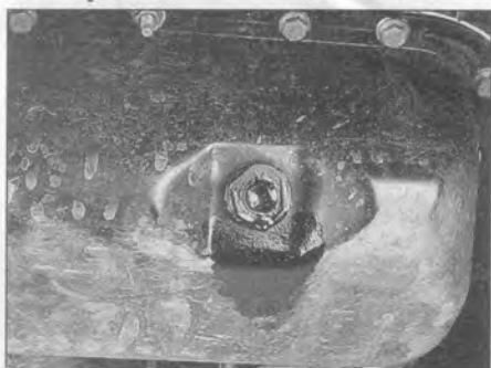
Engine oil may leak from the drain plug...
