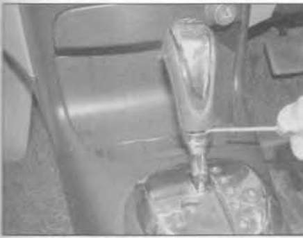
3.2a Carefully prise the selector lever knob locking collar downward to disengage it from the knob ...
