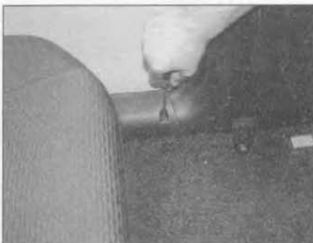
25.21 Undo the screw securing the side trim panel to the base of the centre pillar trim panel – 5-door models
