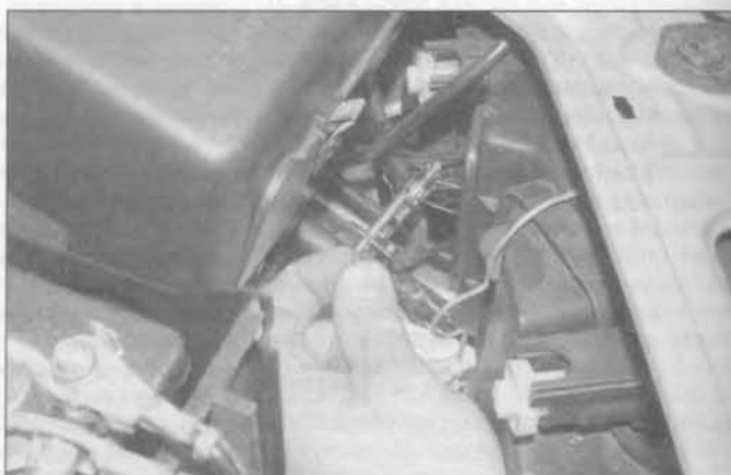
4.5 Release the retaining spring clip and remove the bulb from the headlight unit
