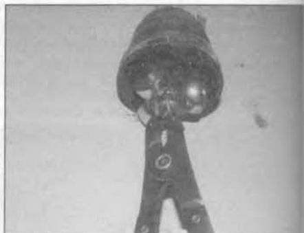
3.22 Using circlip pliers, remove the circlip securing the tripod to the end of the driveshaft
