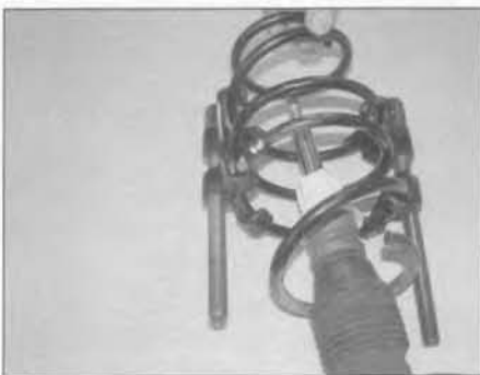
5.4b ... then withdraw the coil spring
