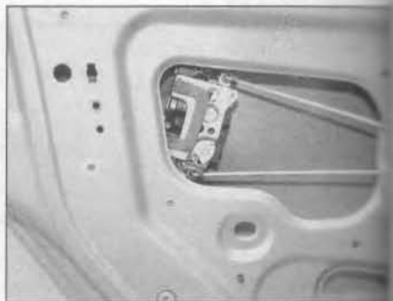
16.45 Manoeuvre the lock mechanism and link rods out through the door aperture
