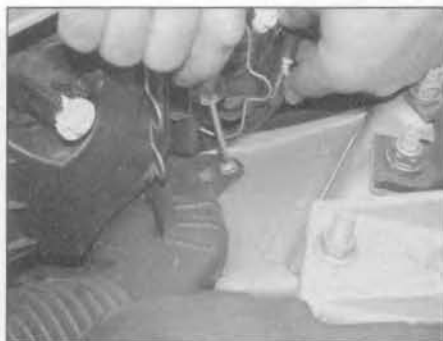
2.11 The cold air intake duct can be removed after undoing the end fitting retaining screw
