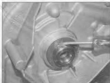
9.2 Carefully prise the crankshaft right-hand oil seal from the oil pump casing
