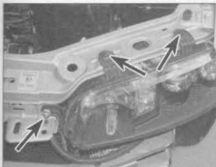
6.2 Unscrew the headlight side and upper securing bolts (arrowed)
