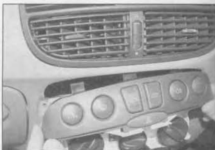
27.21 Lower the panel to free the upper retaining tags, then disconnect the wiring connectors
