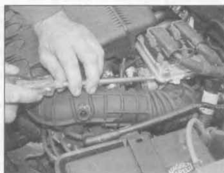
2.7 Release the clips securing the inlet duct to the air cleaner and throttle body
