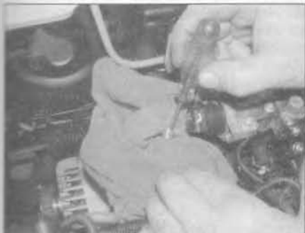
5.6 ... then depress the central plunger to allow the fuel pressure to be released
