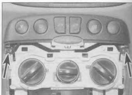
27.20 Undo the two lower screws (arrowed) securing the centre switch panel to the fascia
