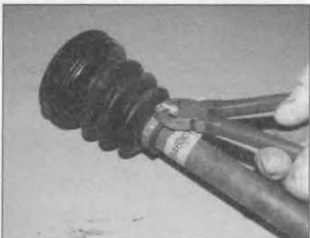
3.20 Release the smaller clip on the inner joint gaiter by cutting it off with side-cutters
