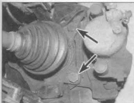
2.5a Undo the brake caliper mounting bracket retaining bolts (arrowed) . . .
