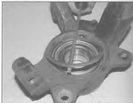
3.5 Extract the bearing retaining circlip from the swivel hub
