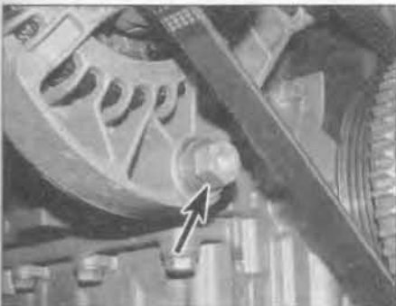
5.5a Slacken the alternator lower pivot bolt (arrowed) . . .
