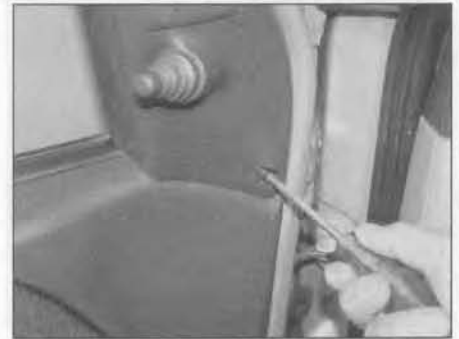
14.1b . . . and undo the screw securing the exterior mirror inner trim panel to the front door
