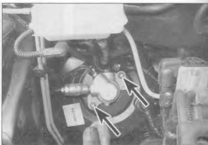
10.5 Master cylinder retaining nuts (arrowed)
