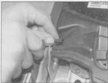
22.4 . . . release the end of weatherstrip from its location each side . . .
