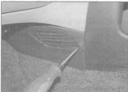
27.14a Undo the retaining screws securing the vent panels to the lower centre panel ...
