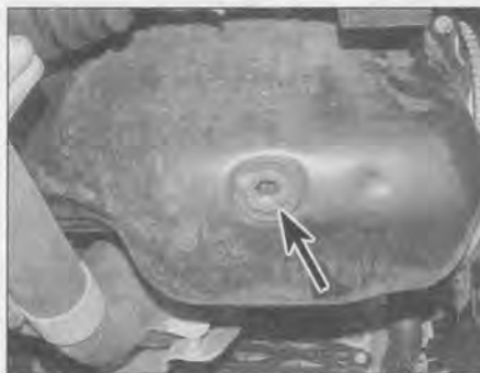
3.3 Engine oil drain plug location (arrowed)
