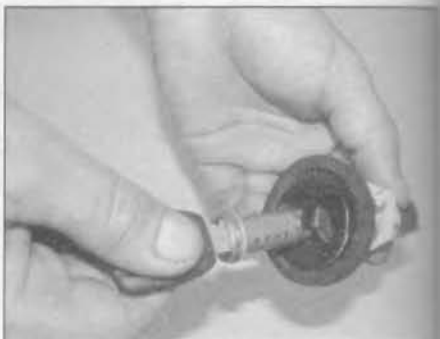
10.8b ... then withdraw the lock barrel from the lock cylinder
