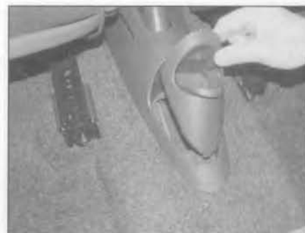
12.9 Undo the retaining screw and remove the ashtray surround
