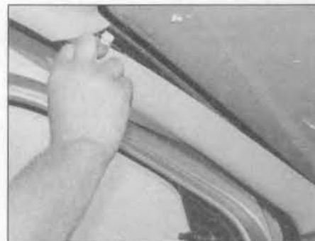
25.10 Carefully pull the front pillar trim panel away from the pillar to release the securing clips
