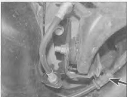
7.4a Release the handbrake cables from their clips on the rear axle mountings (arrowed) . . .
