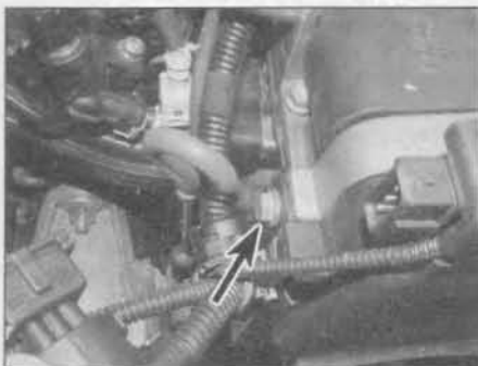
4.9a Undo the retaining bolt (arrowed) at the rear of the upper timing cover ...
