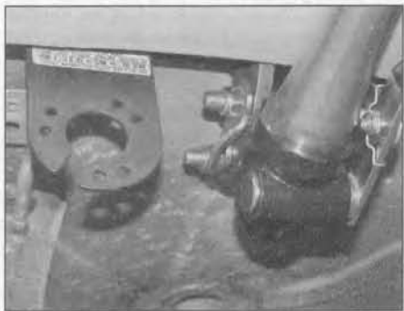
28.18b ... then secure the assembly with the two Nyloc nuts
