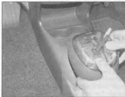
3.3 Release the selector lever cover from the console and lift the cover off the selector lever
