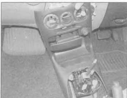
27.17 Disconnect the wiring connector, then withdraw the panel from the fascia
