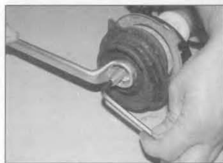
5.3 Unscrew the nut securing the strut piston rod to the upper mounting
