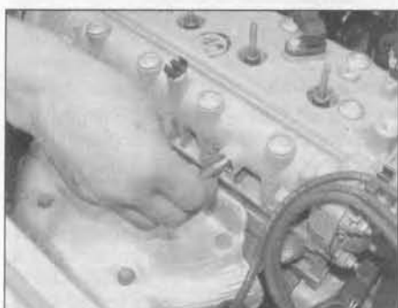
5.15a Screw the camshaft locking tools into the timing holes in the front ...
