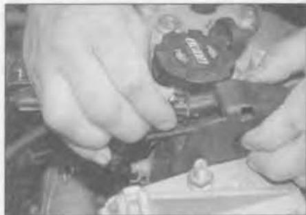
4.4 Disconnect the TDC sensor wiring connector, then release the wiring socket from the clip on the timing cover
