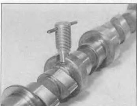
5.15c The tools engage in the camshaft slots when fitted (shown removed for clarity)
