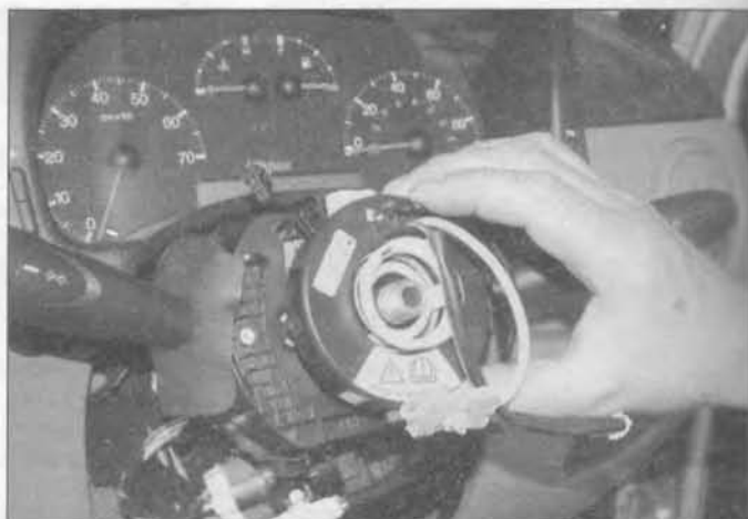
20.13b ... and withdraw the clockspring from the steering column
