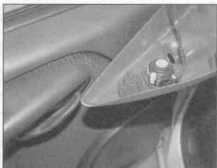
14.3 Pull the mirror trim panel from its location and disconnect the loudspeaker wiring connector
