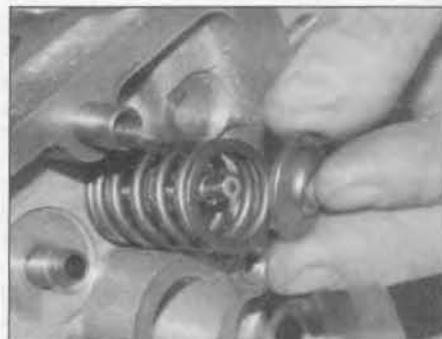
6.7a Release the compressor, and remove the spring retainer ...
