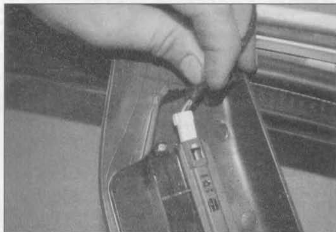
4.41 Withdraw the light unit and disconnect the bulbholder wiring connector
