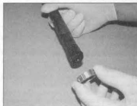
3.11a Slide the smaller garter securing clip onto the driveshaft ...
