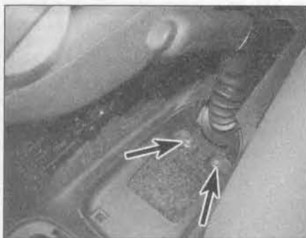
26.4 Undo the two retaining nuts (arrowed) in the oddments tray aperture – manual transmission models
