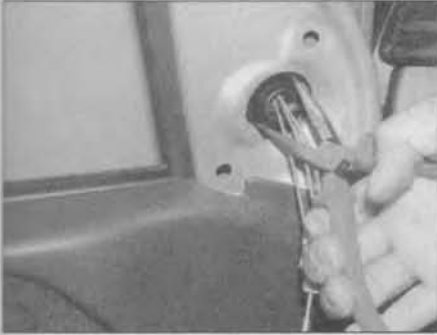
17.4 Using pointed-nose pliers, unscrew the retaining nut and withdraw the mirror from the door
