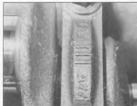
10.5 Main bearing cap identification markings – SOHC (8-valve) engines
