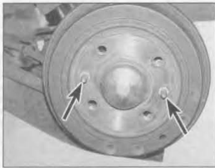
7.2 Slacken and remove the two brake drum locating studs (arrowed)
