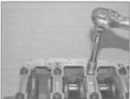
17.16b Tighten the ten inner lower crankcase bolts to the Stage 1 torque setting using a torque wrench ...
