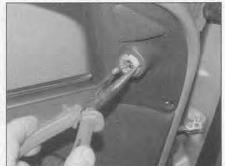
14.2b Using pointed-nose pliers, unscrew and remove the locking collar
