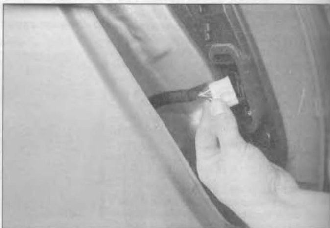
4.32 Withdraw the light cluster and disconnect the wiring connector
