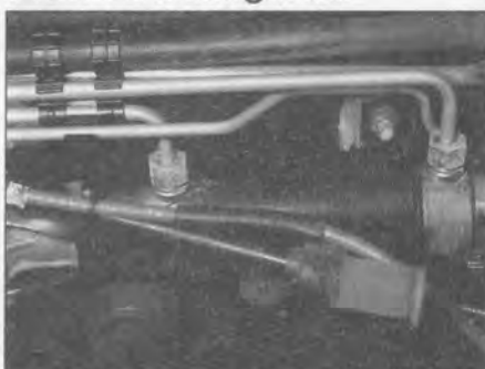
Power steering fluid may leak from the pipe connectors on the steering rack.
