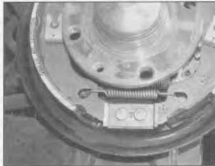
8.5b ... and lower return spring
