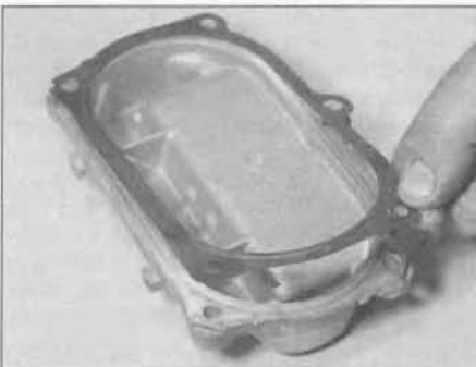
10.20a Locate a new gasket on the cylinder head extension end cover ...
