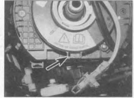
11.7 Check that the clock spring centre position indicator window (arrowed) is centred over the red indicator tab
