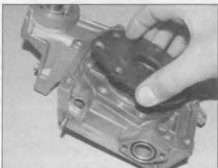
15.9 Extract the fixing screws and remove the oil pump rear cover plate
