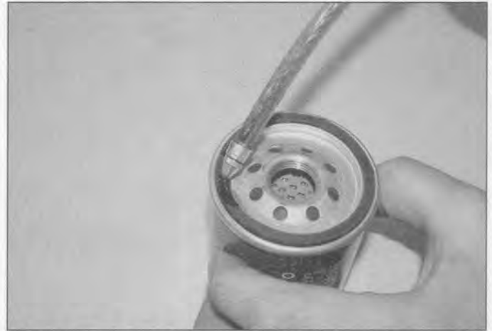
3.9 Apply a light coating of clean engine oil to the sealing ring on the new filter
