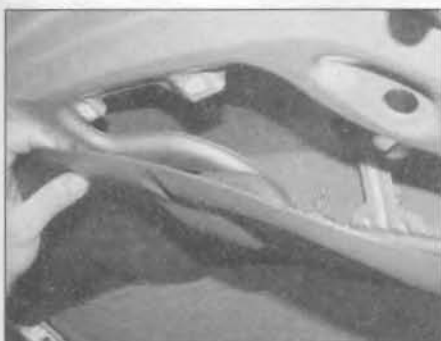
25.4 Pull the panel downwards to release the securing clips, then remove the panel from the tailgate
