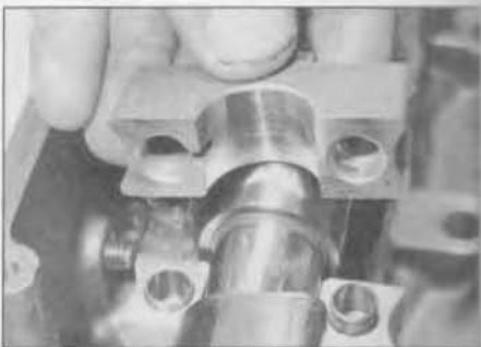
10.6c When removing the camshaft bearing caps, note the position of the long and short locating dowels
