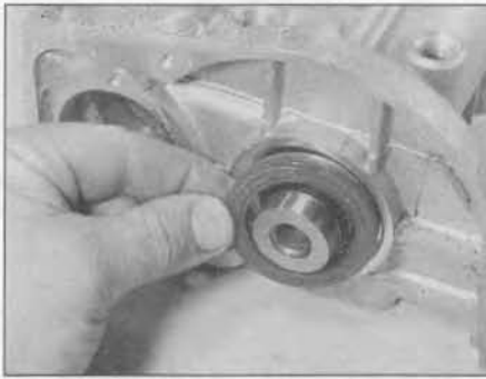
10.16 Fit a new exhaust camshaft oil seal
