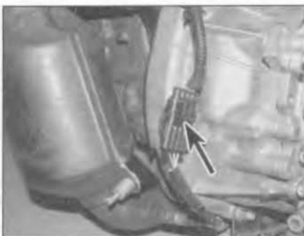
12.6b Downstream lambda sensor wiring connector (arrowed)
