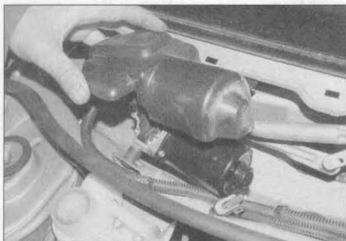
16.4a Lift off the wiper motor protective cover . . .
