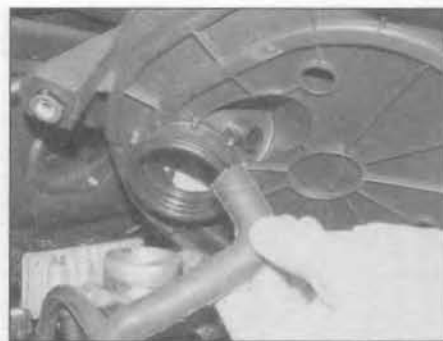
2.4 Lift the air cleaner casing off the throttle body and disconnect the crankcase ventilation hose
