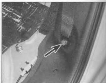
24.22b . . . and lower anchor bolt (arrowed) - 5-door models
