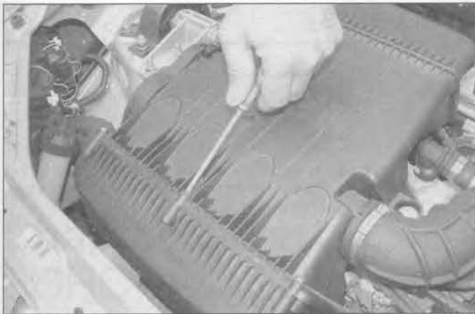
22.5a Undo the bolts securing the air cleaner cover to the main body...
