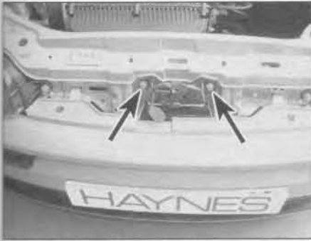
12.3 Bonnet lock assembly retaining nuts (arrowed)
