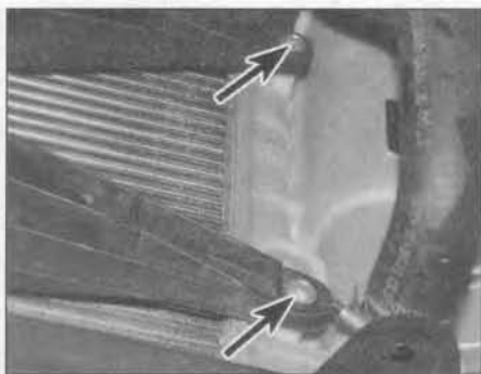
5.10a Undo the bolts (arrowed) securing the fan shroud to the right-hand ...
