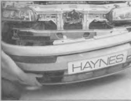
6.8 Carefully withdraw the bumper from the car
