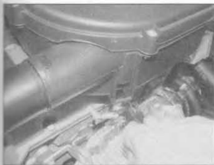
2.2 Release the spring-tensioned clasp at the front of the air cleaner casing
