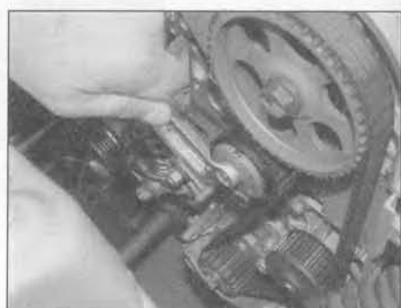
5.16 Release the nut on the timing belt tensioner ...
