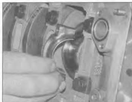
9.6 Unscrew the retaining bolts and remove the big-end cap and bearing shell
