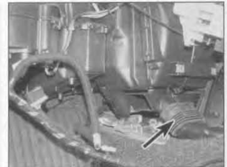
8.8 Remove the rubber sleeve (arrowed) between the heater and floor air ducts
