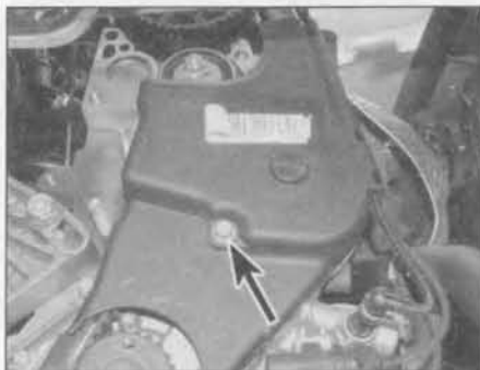
4.15 Undo the retaining bolt (arrowed) in the centre of the lower timing cover
