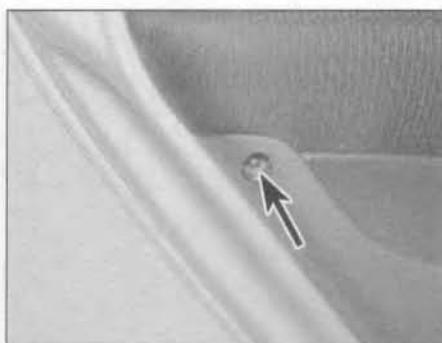
14.17b ... and undo the screw (arrowed) securing the rear of the trim panel to the door
