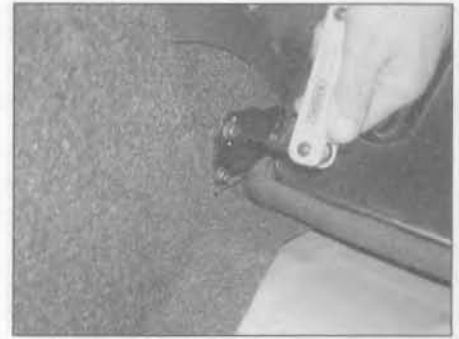
23.8 Undo the two side hinge securing bolts and remove the seat back from the car
