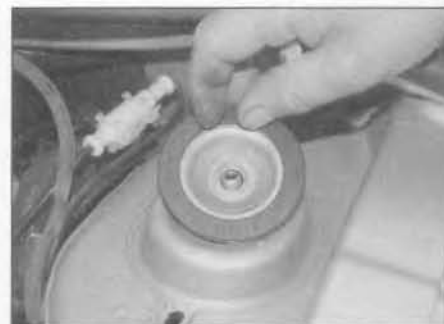
4.5b ... lift off the mounting cup and withdraw the strut from under the wheel arch
