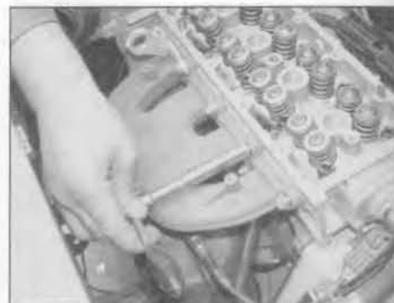
11.4 Undo the retaining nuts and withdraw the exhaust manifold off the mounting studs
