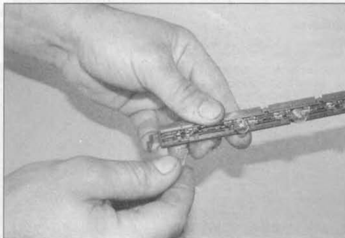
4.43 Remove the relevant push-fit bulb from the bulbholder
