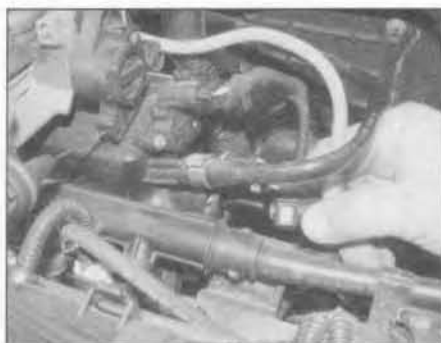
2.6b ... and fuel vapour hose from the control solenoid – SOHC (8-valve) engines
