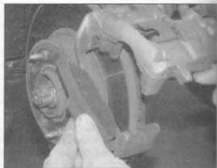
4.4a Pivot the caliper body upwards and withdraw the outer brake pad . . .
