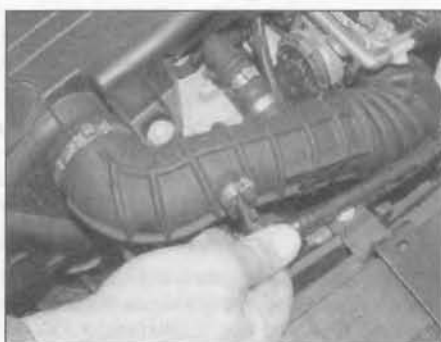
2.6 On DOHC (16-valve) engines, disconnect the vacuum hose from the air cleaner-to-throttle body inlet duct
