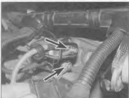
8.6 Unscrew the nuts (arrowed) and disconnect the wiring from the solenoid terminal studs
