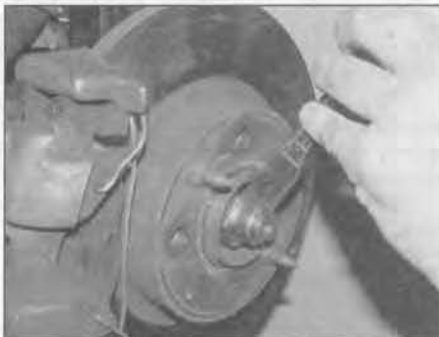
2.19 Secure the driveshaft retaining nut by tapping the staking into the two grooves in the CV joint
