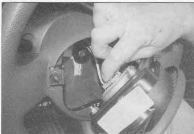
20.5 Lift the airbag unit from the steering wheel and disconnect the wiring connector
