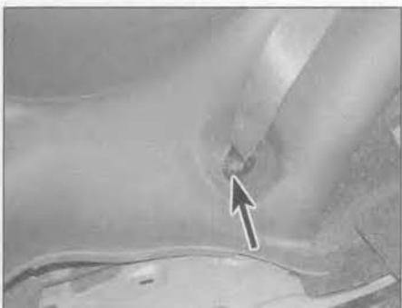
25.33 Undo the rear seat belt lower anchor bolt (arrowed) – 3-door models
