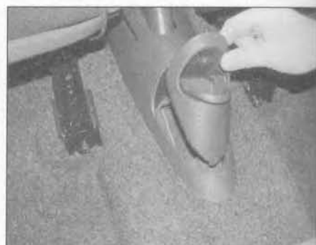
26.6b . . . and remove the ashtray surround from the console – manual transmission models
