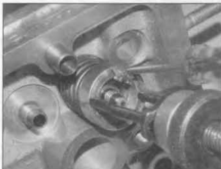
6.6b ... and extract the two split collets from the top of the valve stem
