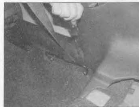
25.6b . . . and rear of the sill trim panel
