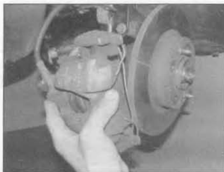
2.5b . . . and withdraw the caliper and mounting bracket assembly off the disc
