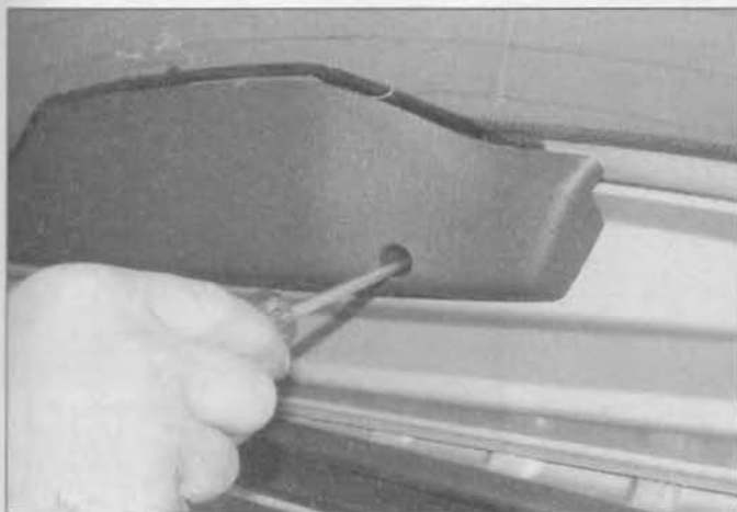
4.40 Undo the two high-level stop-light unit retaining screws
