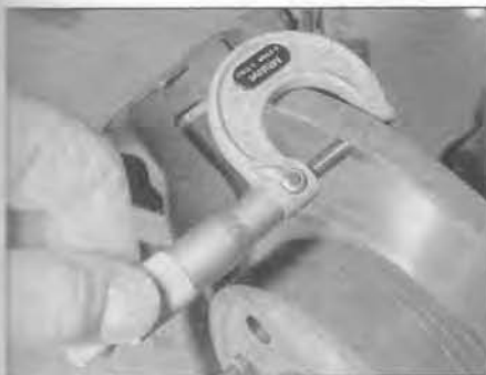
6.8 Measuring brake disc thickness with a micrometer
