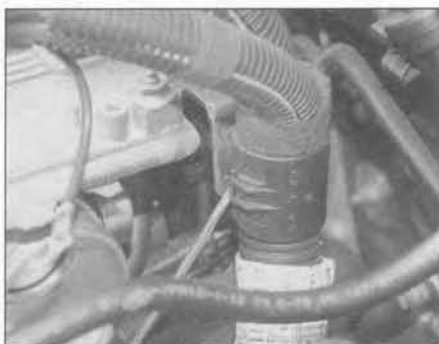
11.24 Open the clip and free the ECU wiring harness from the throttle body – DOHC (16-valve) engines
