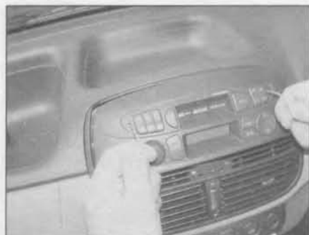
12.2 Remove the radio/cassette player using the special extraction tools
