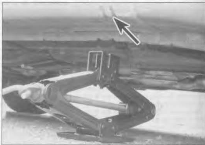
Reinforced jack location points (arrowed) are located at the front and rear of the sills on each side of the car
