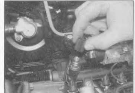
5.5 Withdraw the plastic cap from the top of the Schrader valve...
