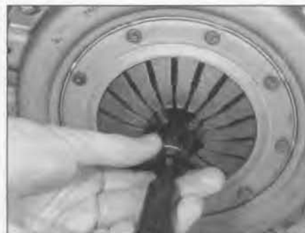
5.16 Using a clutch friction plate centralising tool
