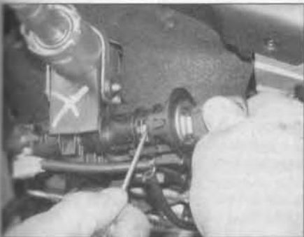
12.4a Depress the release button with a small screwdriver . . .
