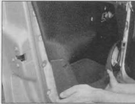
14.10 Using a forked tool, release the press-stud clips, then lift the trim panel from the door
