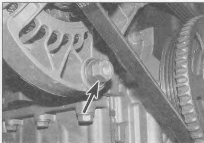
4.7a Alternator lower pivot bolt (arrowed) . . .
