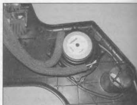
10.10 Disconnect the wiring connectors, undo the screws and remove the speaker
