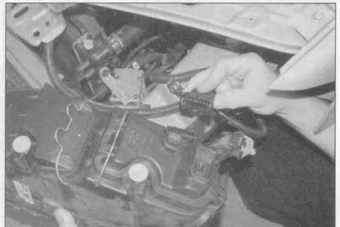
6.4 Disconnect the wiring connector and remove the headlight unit
