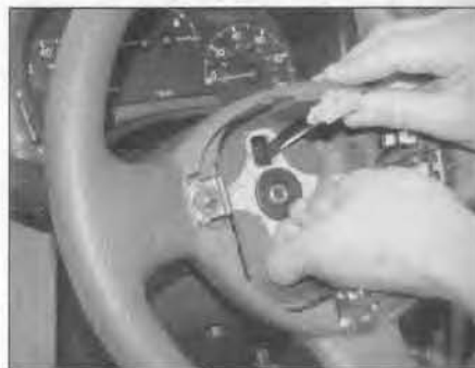
11.3 Lift off the protective seal over the steering wheel retaining nut
