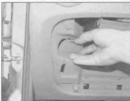
27.38 Prise out the lower retaining bolt access cover on the passenger's side
