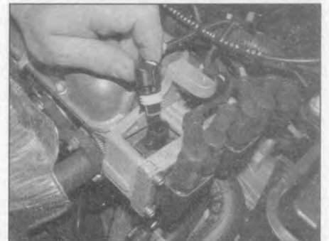
C Check the condition and security of critical wiring connectors such as those at the ignition coils ...
