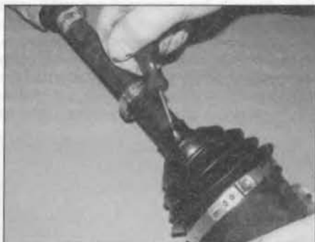
3.16 Lift the lip of the gaiter to expel any air trapped inside
