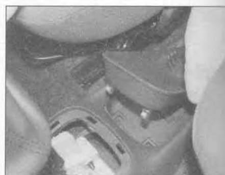
26.3 Carefully prise up the front of the oddments tray to release the two retaining clips – manual transmission models
