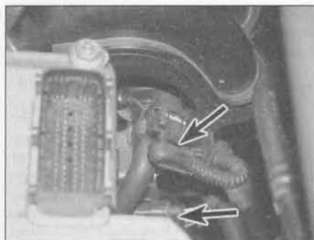
11.25b . . . and at the evaporative emission control solenoid and fuel injector harness (arrowed) – DOHC (16-valve) engines
