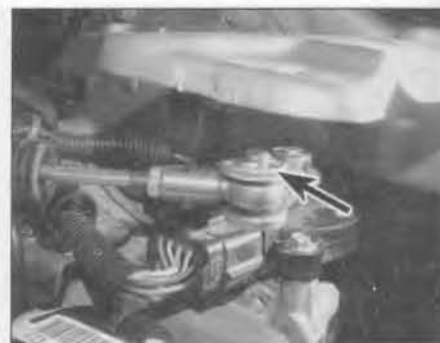
4.13 Extract the retaining clip (arrowed) and release the selector cable end fitting – automatic transmission models
