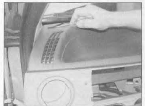
27.36 Carefully prise out the retaining bolt access covers from the top of the facia
