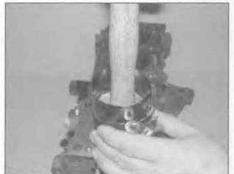
18.9 Tap the assembly into the cylinder using a block of wood or hammer handle
