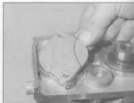
10.5b ... then undo the two bolts and remove the cover plate over the inlet camshaft
