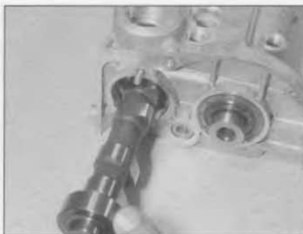
10.9 Carefully remove the inlet camshaft from the cylinder head extension
