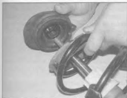
5.4a Withdraw the upper mounting and upper spring seat ...
