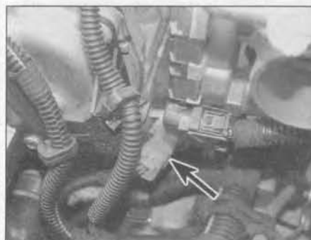
6.1 Engine coolant temperature sensor location (arrowed) on the left-hand end of the inlet manifold
