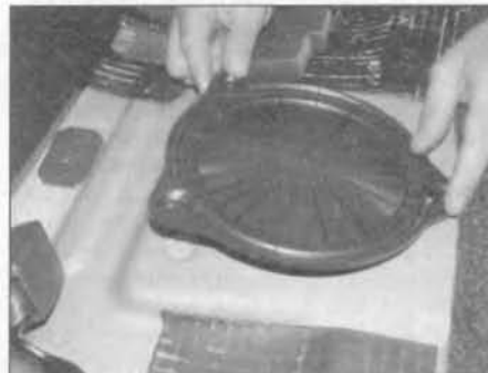
6.4 Remove the fuel pump cover from the aperture in the floor panel
