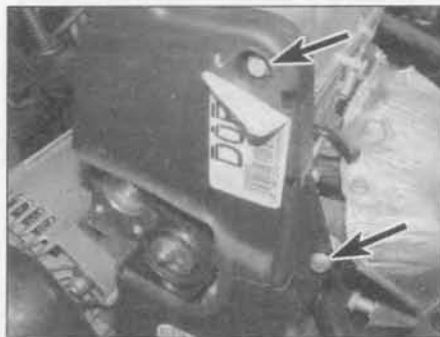
4.9b ... and the upper and lower retaining bolts (arrowed) at the front
