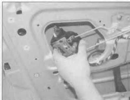
16.26 Manoeuvre the lock mechanism and locking knob link rod out through the door aperture
