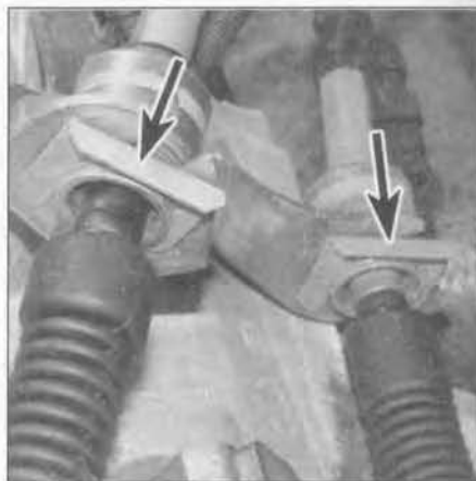
3.3 Extract the retaining clips (arrowed) securing the selector cables to the transmission support bracket
