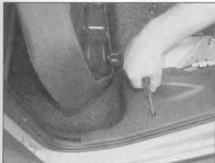
25.42 Undo the screws securing the side trim panel to the sill in the rear door aperture – 5-door models
