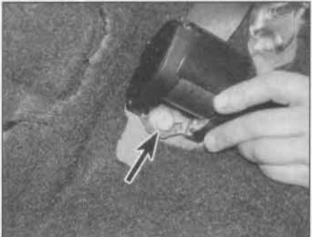
24.25 Rear seat belt inertia reel retaining bolt (arrowed) - 5-door models
