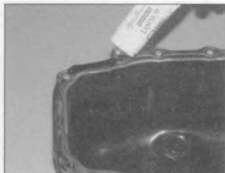
14.7 Apply a 3.0 mm bead of RTV silicone sealant to the sump flange, then locate the sump in position
