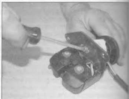
10.7 Undo the screw securing the lock cylinder to the tailgate lock body
