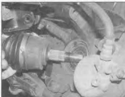
2.7b ... and withdraw the driveshaft outer constant velocity joint from the hub assembly
