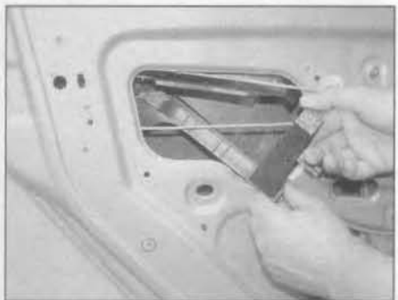
16.40b ... and remove the window glass lower rear guide channel
