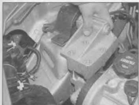
5.8 Undo the retaining nuts and remove the right-hand engine mounting and upper bracket assembly
