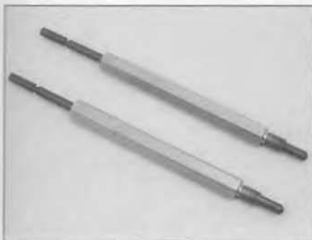
2.2b Fiat special tool for setting piston position ...
