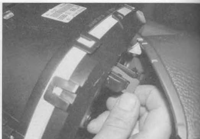
7.5 Lift up the wiring connector locking catch and disconnect the connector
