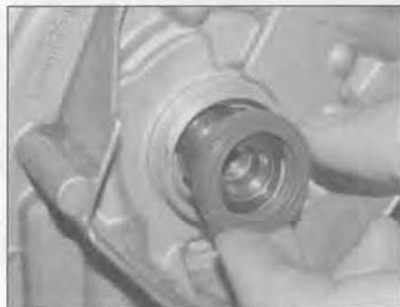
8.4 Locate the new oil seal on the oil pump casing with the sealing lips facing inwards
