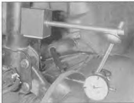
6.11 Using a dial test indicator to measure brake disc runout
