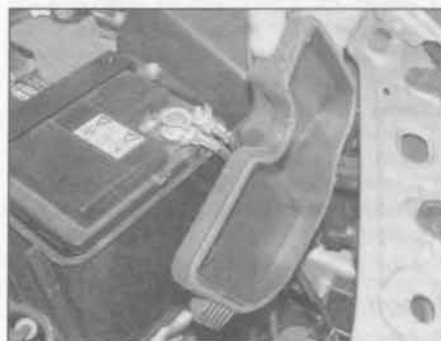
4.8b ... and lift off the plastic cover from the rear inner corner of the headlight unit
