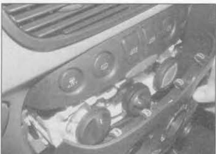
27.16 Carefully prise free the upper edge of the panel to disengage the four retaining clips
