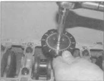
17.16c ... then through the Stage 2 angle using an angle-measuring gauge - DOHC (16-valve) engines
