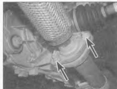
12.7 Exhaust system front pipe flange retaining nuts (arrowed)
