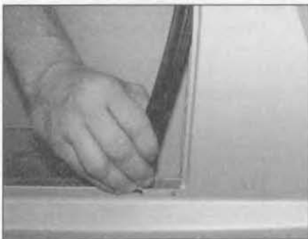
18.25 Lower the glass to the bottom of the guide channels, and pull the rear channel out of the door aperture
