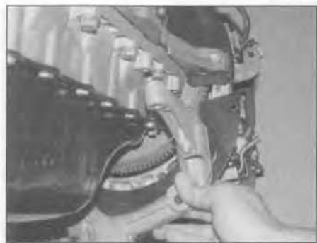
14.3 Undo the bolts and remove the support brace linking the transmission to the cylinder block
