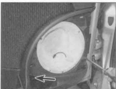
14.6 Undo the three retaining screws in the loudspeaker aperture, and the single screw (arrowed) in the oddments pocket
