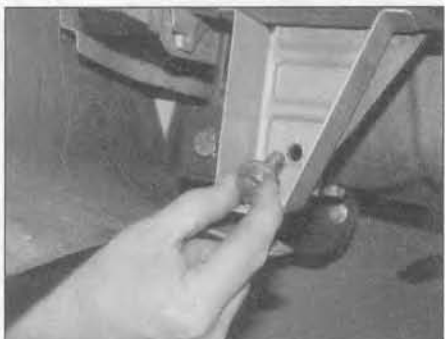
28.19b ... fit the mounting bolts with a flat washer under the bolt head and secure with the nuts and lockwashers
