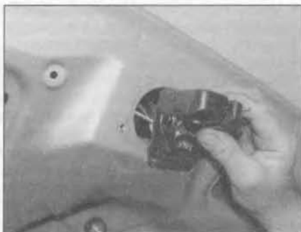
10.4 ... and withdraw the tailgate lock assembly, together with the lock cylinder
