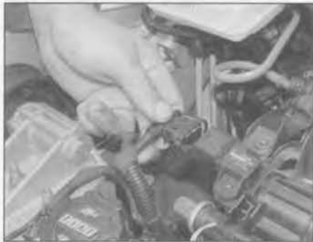
10.21 Disconnect the wiring connector at the intake air temperature/pressure sensor
