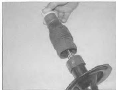
5.5 Release the dust cover from the strut body, then withdraw the dust cover and bump rubber
