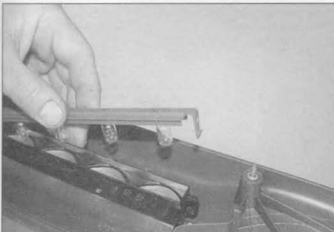
4.42 Release the plastic retaining clip and lift the bulbholder from the light unit
