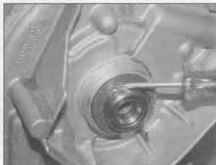
8.2 Carefully prise the crankshaft right-hand oil seal from the oil pump casing
