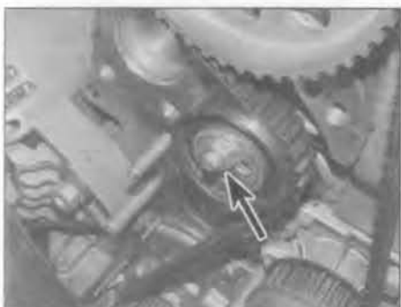
5.5 Undo the nut (arrowed) and move the timing belt tensioner pulley away from the belt
