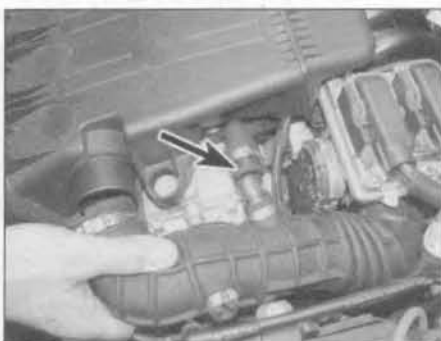
2.8 Release the clip, disconnect the breather hose (arrowed) and lift out the inlet duct
