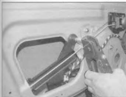
16.8 Refit the anti-theft partition and secure with new pop rivets
