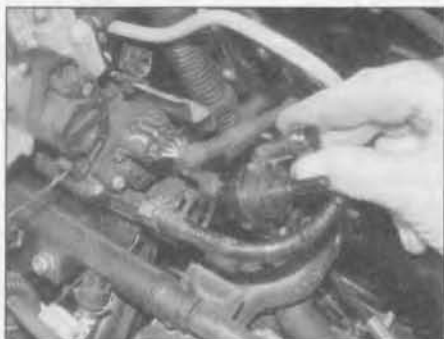
2.7b ... and remove the solenoid from the inlet manifold – SOHC (8-valve) engines
