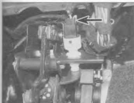
11.4 Stop-light switch wiring connector (arrowed)
