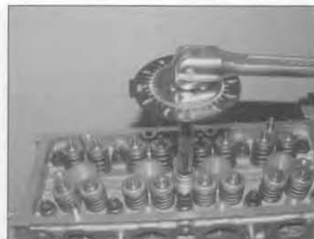
11.17c ... then through the Stage 2 and Stage 3 angle
