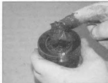
3.12 Pack the joint with the specified grease, then twist the joint to ensure all recesses are filled
