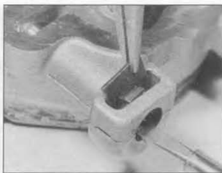
15.8a Removing the oil pump pressure relief valve keeper plate
