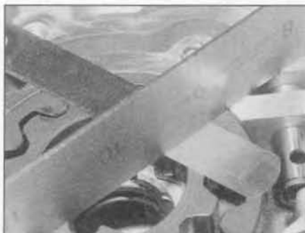
15.11b Measuring oil pump rotor endfloat
