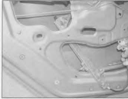
18.37 Disengage the regulator shaft, then manipulate the regulator assembly out through the door aperture
