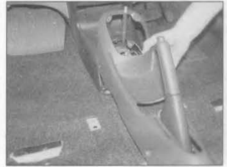
26.18 Lift the console from its location and remove it from the car – automatic transmission models
