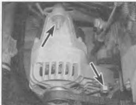
5.5b . . . and upper adjustment bolts (arrowed), then swivel the alternator towards the engine to remove the drivebelt
