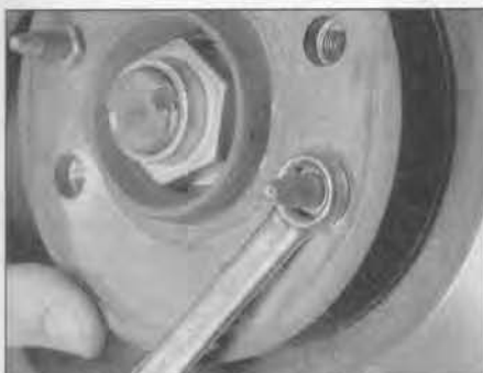
6.18a Remove the disc locating studs . . .
