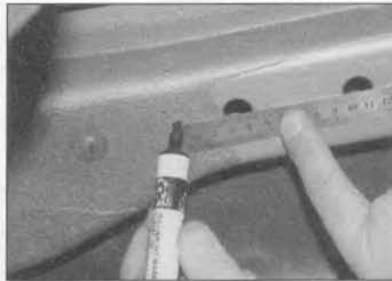
28.11 Mark the chassis side rail 35.0 mm forward from the centre of the forward-most mounting hole
