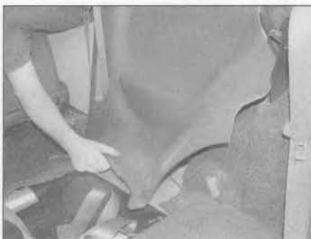
25.35 Carefully pull the side trim panel away from the body to release the securing clips – 3-door models
