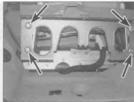
20.19 Undo the bolts (arrowed) securing the airbag assembly to the fascia rail
