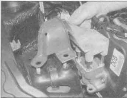
4.5 Undo the retaining nuts and lift the right-hand engine mounting and upper bracket assembly off the studs
