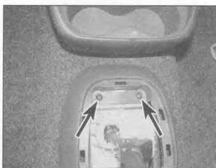
26.2b . . . then undo the screws (arrowed) securing the console to the gear lever housing – manual transmission models
