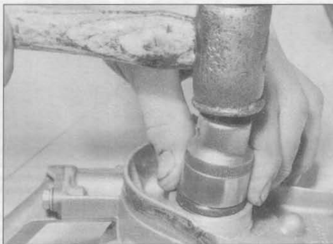
15.15b Using a socket to fit a new oil seal to the oil pump
