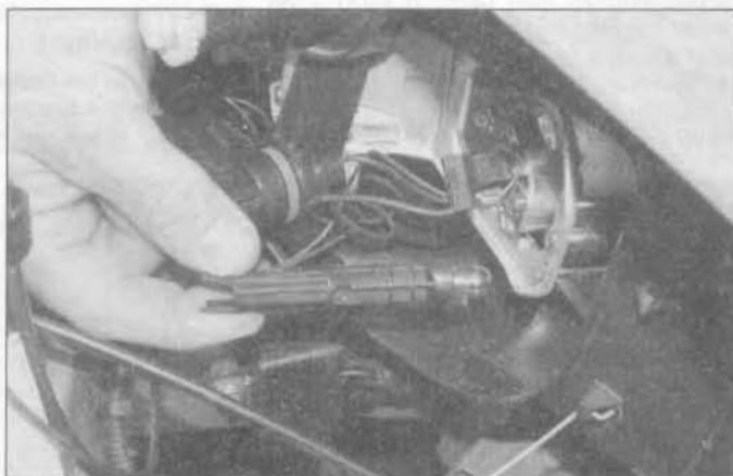
4.15 Depress the retaining tabs and withdraw the sidelight bulbholder from the headlight unit
