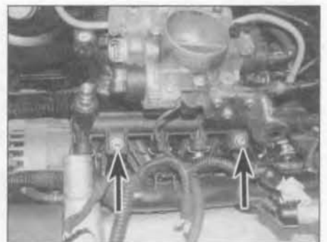
9.14 Unscrew the two bolts (arrowed) securing the fuel rail assembly to the inlet manifold
