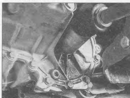
Gearbox oil can leak from the seals at the inboard ends of the driveshafts.
