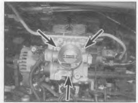
9.7 Throttle body retaining bolts (arrowed)
