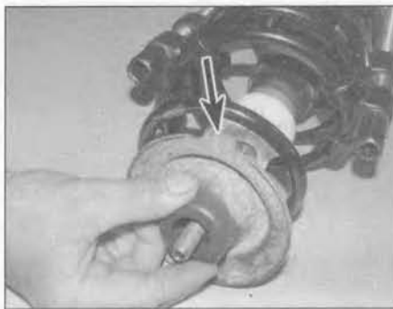
5.11a Locate the upper spring seat over the piston rod, ensuring that the raised projection (arrowed) . . .
