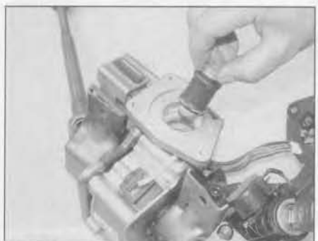
14.3 Remove the drive coupling from the gearbox
