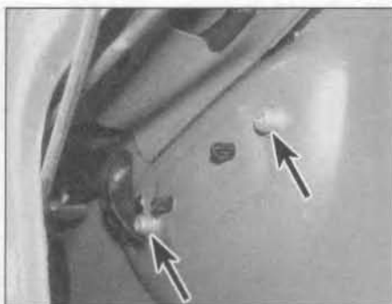
16.31 Undo the two exterior handle retaining bolts (arrowed) and withdraw the handle from the door
