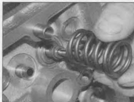
6.7b ... and valve spring
