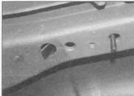
28.12c ... Feed the strap through the chassis side rail, allowing the mounting stud to protrude through the existing hole
