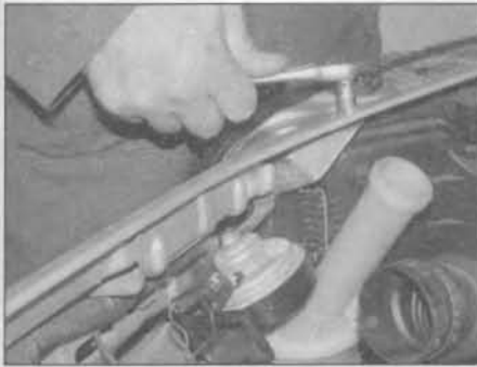
9.2 Undo the bolt securing the horn mounting bracket to the front body panel
