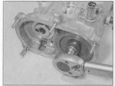
10.17 Tighten the inlet camshaft drivegear retaining bolt to the specified torque
