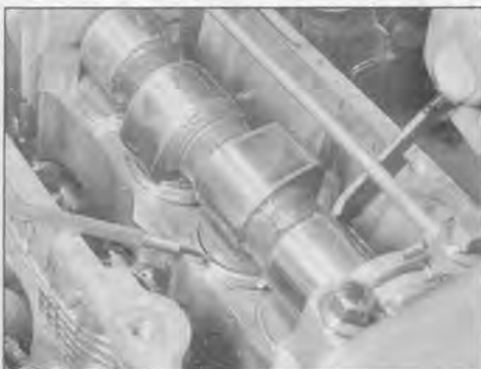
15.11 Using a modified C-spanner and a screwdriver to remove a shim
