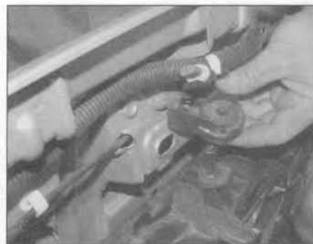
5.9b ... and remove the upper mounting bracket from the top of the fan shroud
