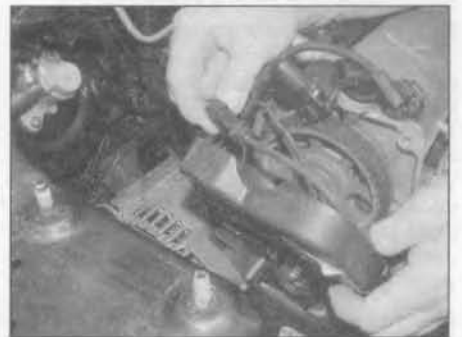
4.10 Lift the cover upwards and slip the wiring out of the groove in the cover periphery
