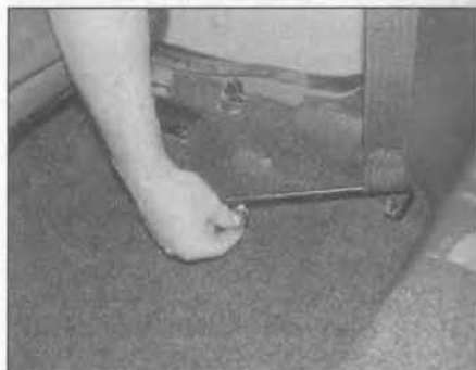
25.32 Undo the bolt securing the front seat belt lower anchor rail to the base of the sill – 3-door models
